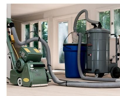
A PROPER DUSTLESS SET-UP There are new dustless sanding systems that retro-fit to sanding equipment allowing the hardwood restoration process to be almost dust free.
